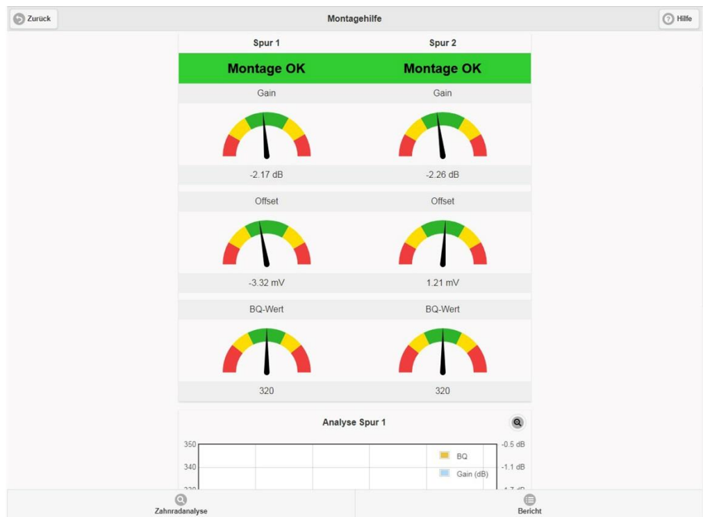
Figure 3: Mounting aid in the web browser: If all displays are in the green range, the sensor is fitted correctly
