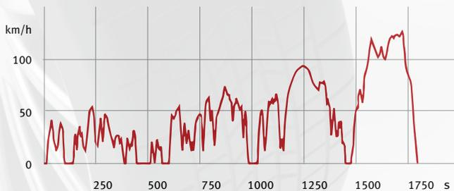
Driving cycle for the "Worldwide Harmonised Light Vehicles Test Procedure" (WLTP)
