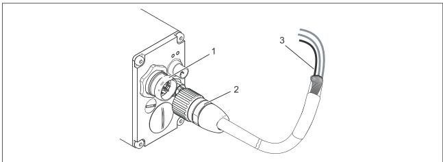
Power supply cable BZK23**S1**A\_ \_ L
