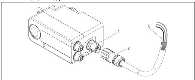
Power supply cable BZK17**S1**A\_ \_ L
