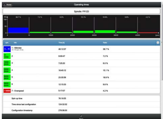
Operating time in different rotational speed ranges Visualization of configurable operating hours meter in the MiniCODER with optional extras P
